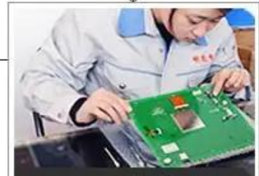
Install the motherboard
